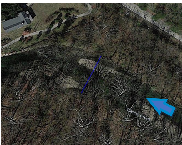
Site 46, upstream of Castle and Key Distillery and downstream of Millville was positioned across a small island to allow for wading while also measuring perpendicular flow.
